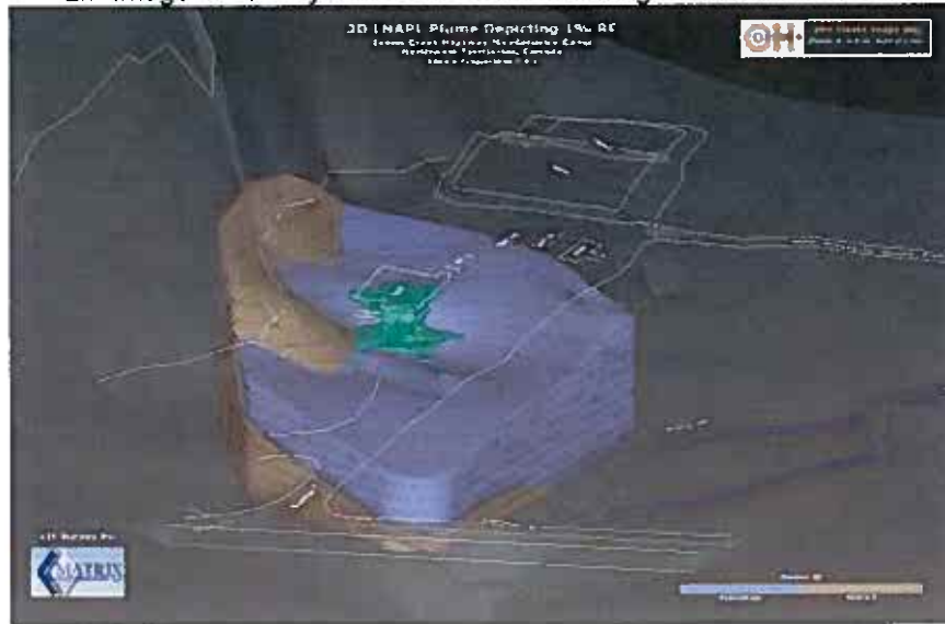
LIF Image 4: 3D Hydrocarbon Plume Showing Permafrost and Bedrock
