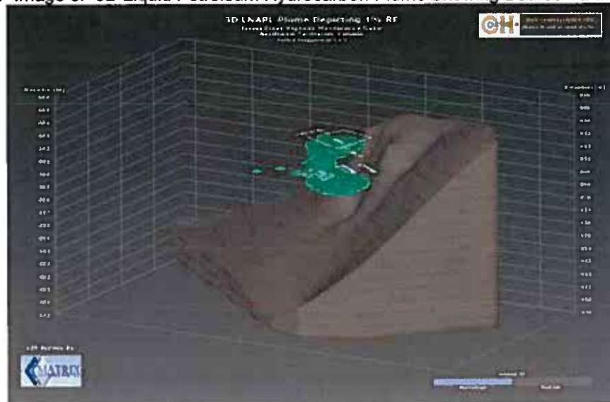
LIF Image 5: 3D Liquid Petroleum Hydrocarbon Plume Showing Bedrock Surface
