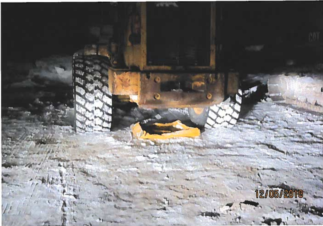
Figure 2 drip tray put in place
