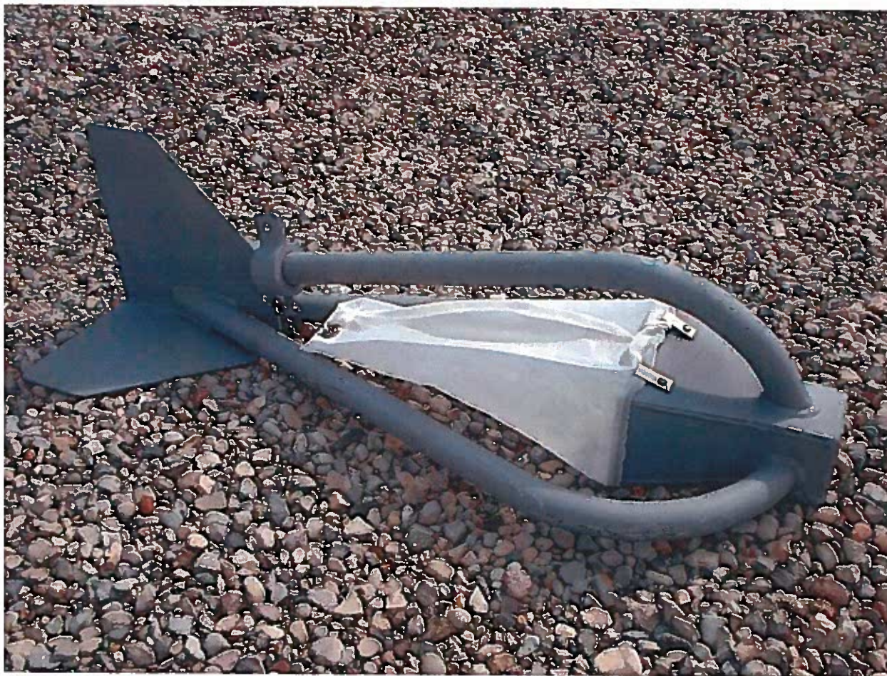
Figure 3. A Helley-Smith suspended sediment sampler. The sampler is deployed near the streambed and moving sediments are captured in the filter screen. The deployment of the sampler is timed so that quantitative estimates of bedload movement can be obtained.
