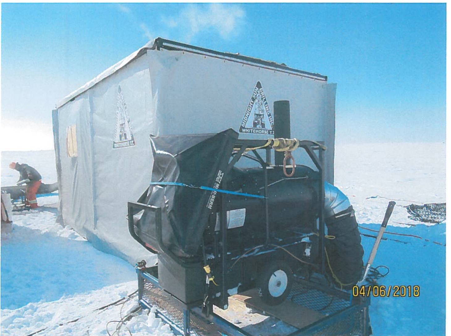
Photo #6 - MV2012C0009 - Dominion Diamond Mines ULC Heater had secondary containment present.
