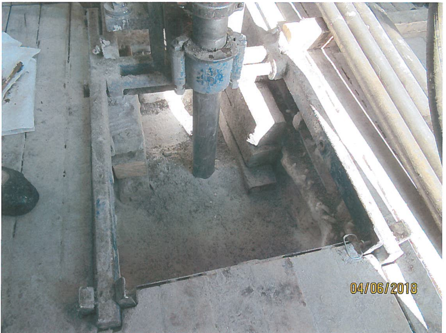
Photo #2 - MV2012C0009 - Dominion Diamond Mines ULC View of the RC drill collar. Drill cuttings are being contained at the collar with a snow berm.
