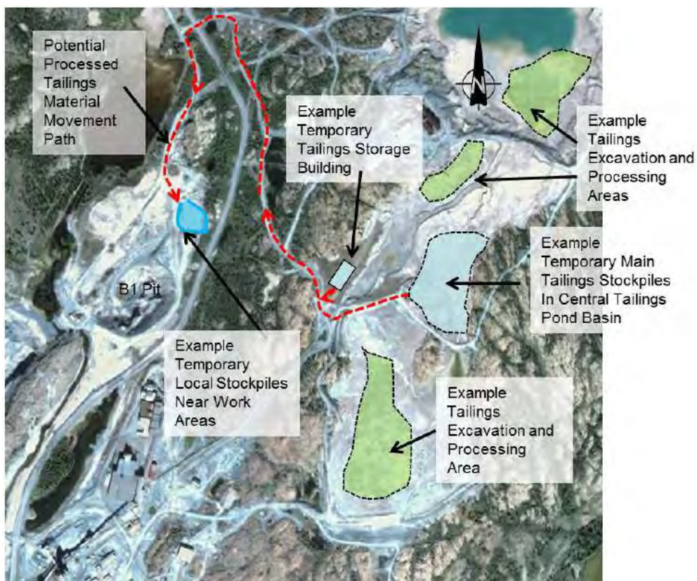
Figure 3 – Example Tailings Excavation, Processing, Storage and Haulage Path (CARD, 2017)
