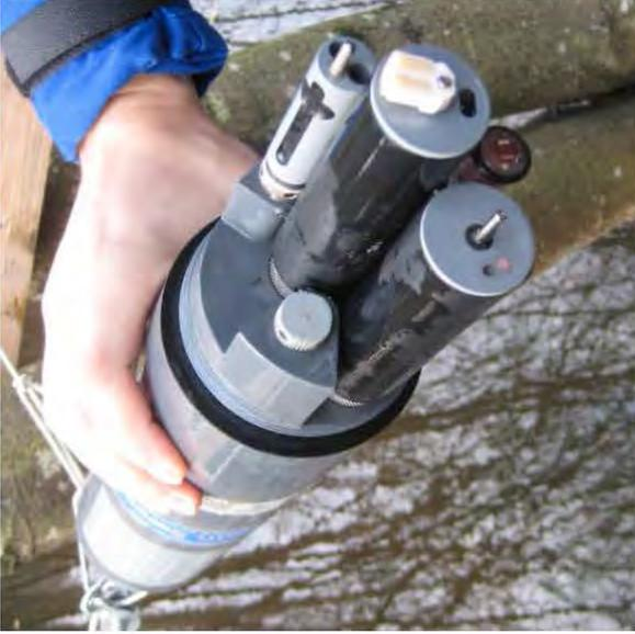
**YSI 6600 Sonde with Fluorometer**
