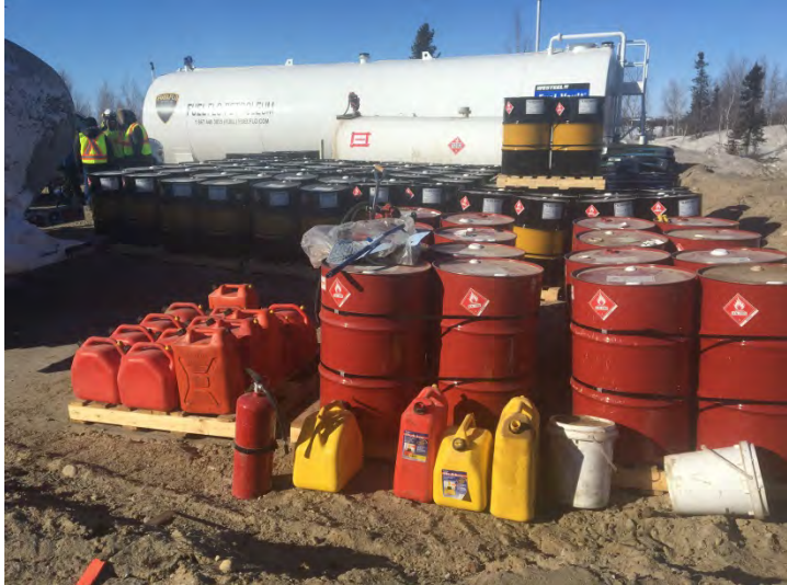
Photo #8: Fuel Berm at Camlaren mine containing 50 drums of premium gasoline. 16 drums of regular gasoline. 108 drums of Jet A fuel, for helicopter work in the summer
