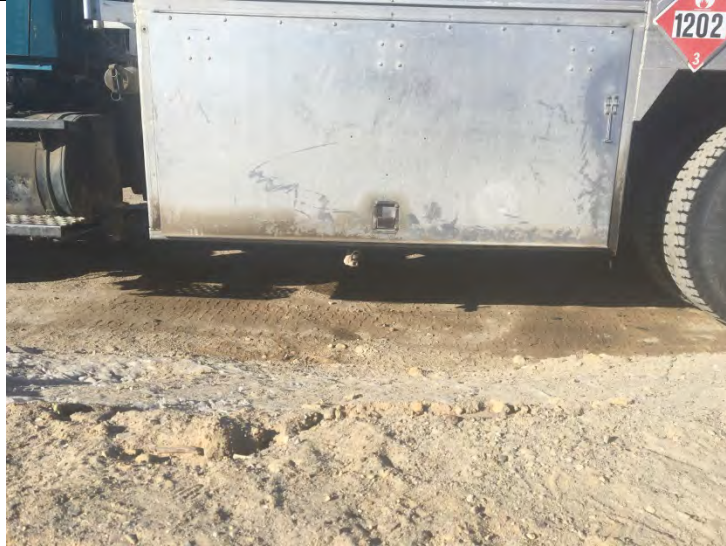
Photo #10: Fuel Truck with a small leak resulting in staining of coil underneath.
