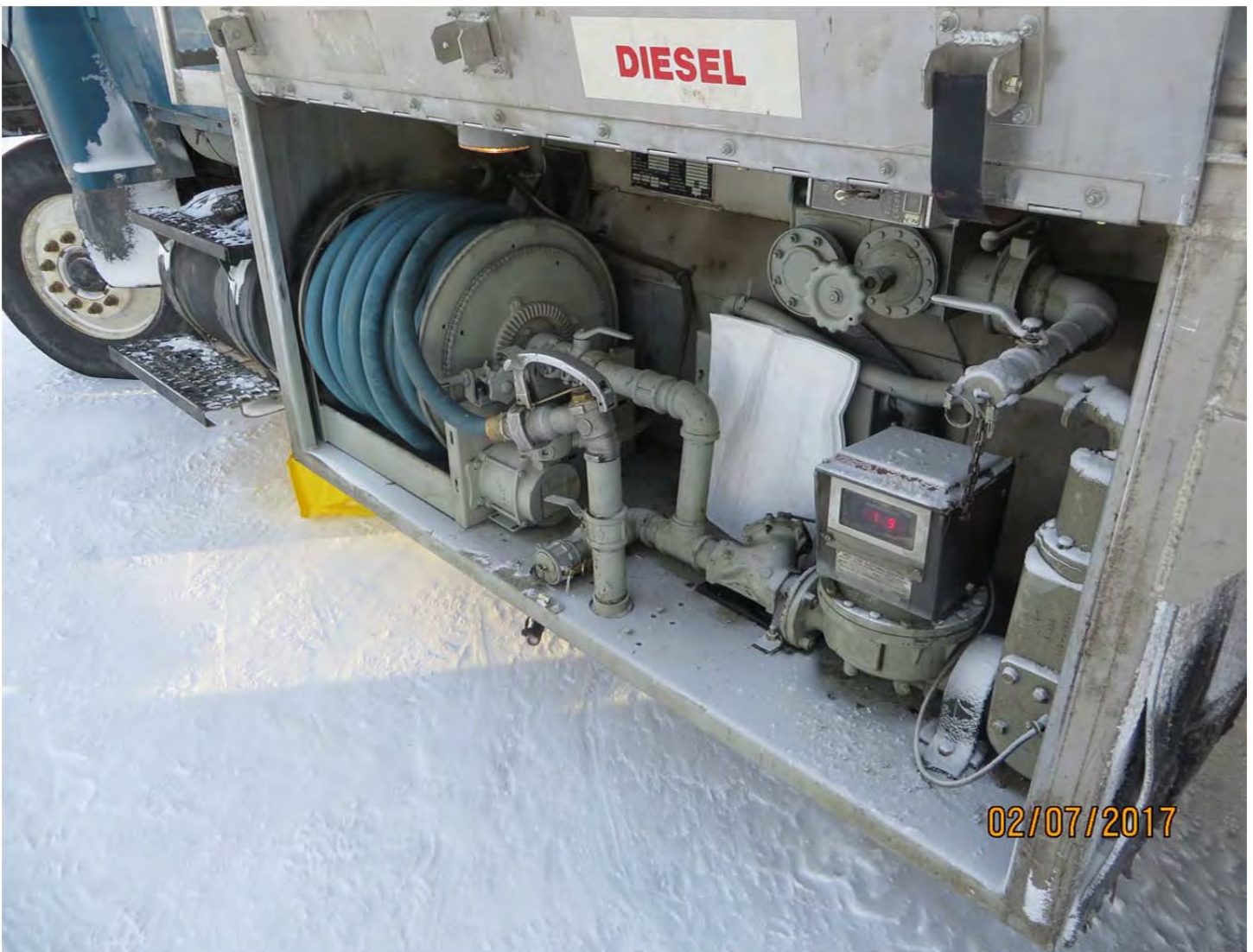
Photo #3 - MV2016X0011 - INAC-CARD - Tundra No obvious hydrocarbon leaks or spills were observed in the dispensing compartment of the fuel truck.
