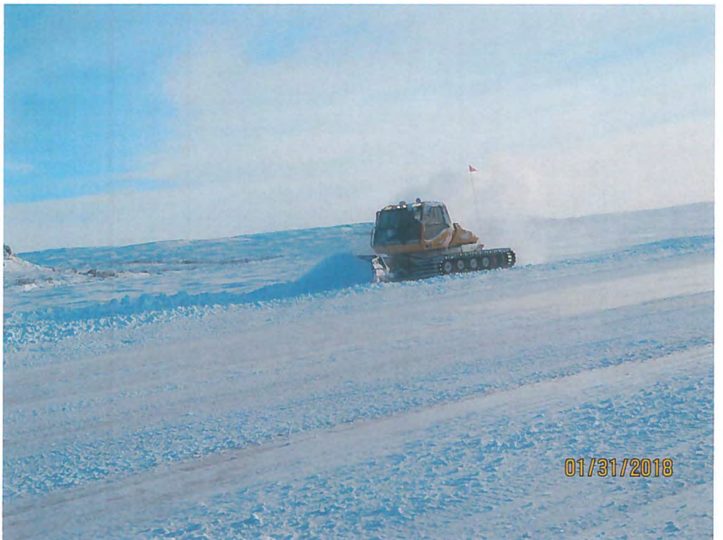
Photo #4 - MV2016X0011 - INAC-CARD - Tundra Mine Snowcat actively knocking down the windrows on the ice surface of Mackay Lake.
