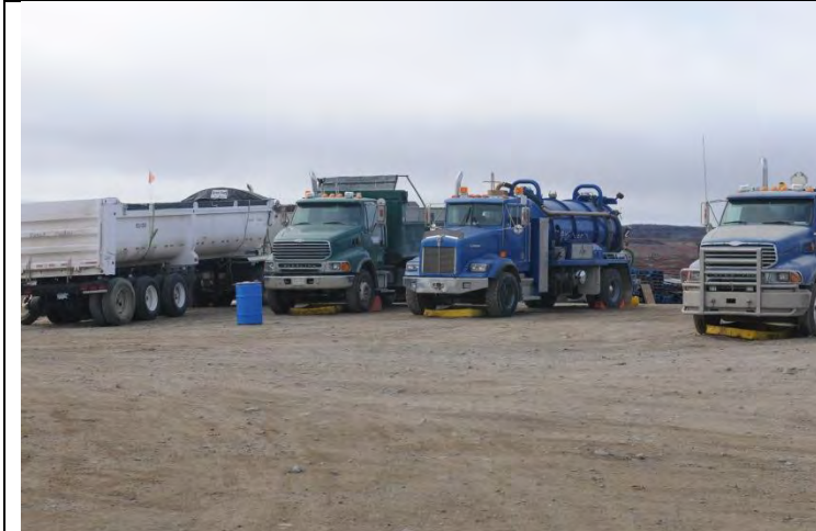
Photo #7: Drip trays placed under vehicles that were parked for over 2 hours.
