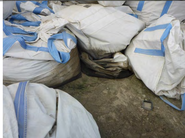
Photo #6: Stains on the bags in the Hazardous lay down area from a previous spill.
