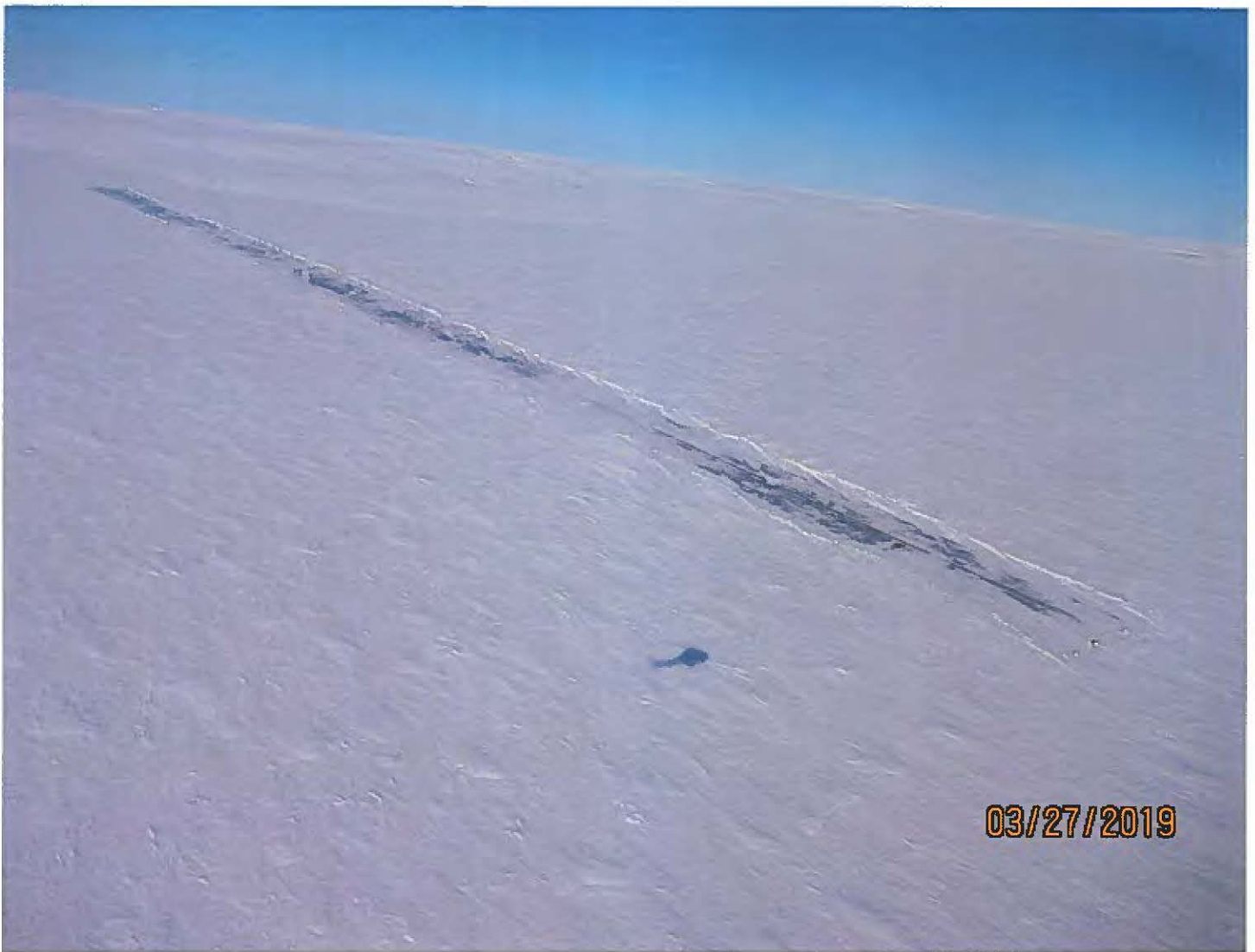
Photo #1 - MV2017C0022 - Glowworm Lake An airstrip was cleared on the ice surface of Glowworm Lake to accommodate the use of a Dash 7 aircraft for fuel delivery.
