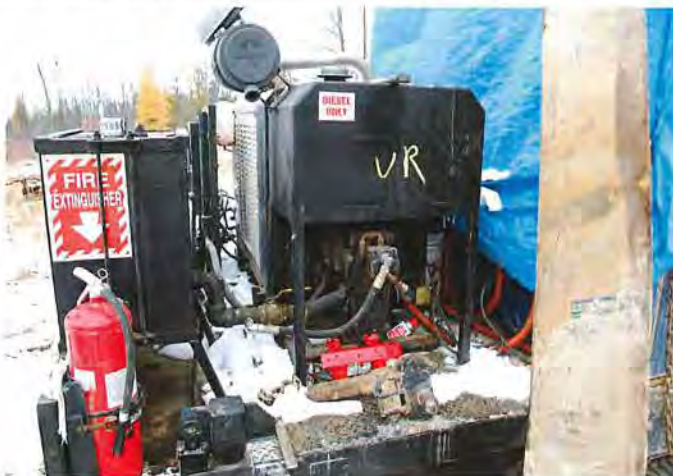
Figure 5 Close up of hydraulic tank on left and diesel tank on right.
