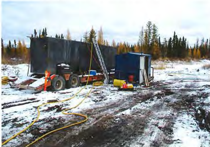
Figure 3 Drill with drip tray under it.
