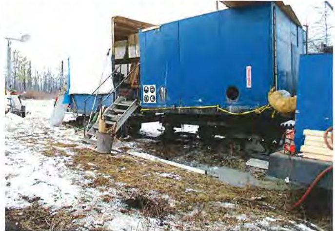
Figure 4 Tanks on drill unit no secondary containment.
