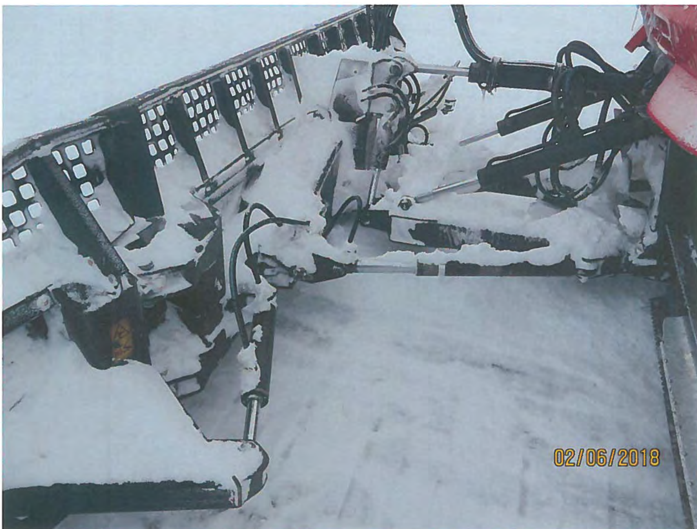
Photo #4 - MV2017X0005 - NTPC - Bluefish Winter Road No hydrocarbon leaks of concern were noted on the blade of the snowcat. When possible, fittings are wrapped with absorbent matting.
