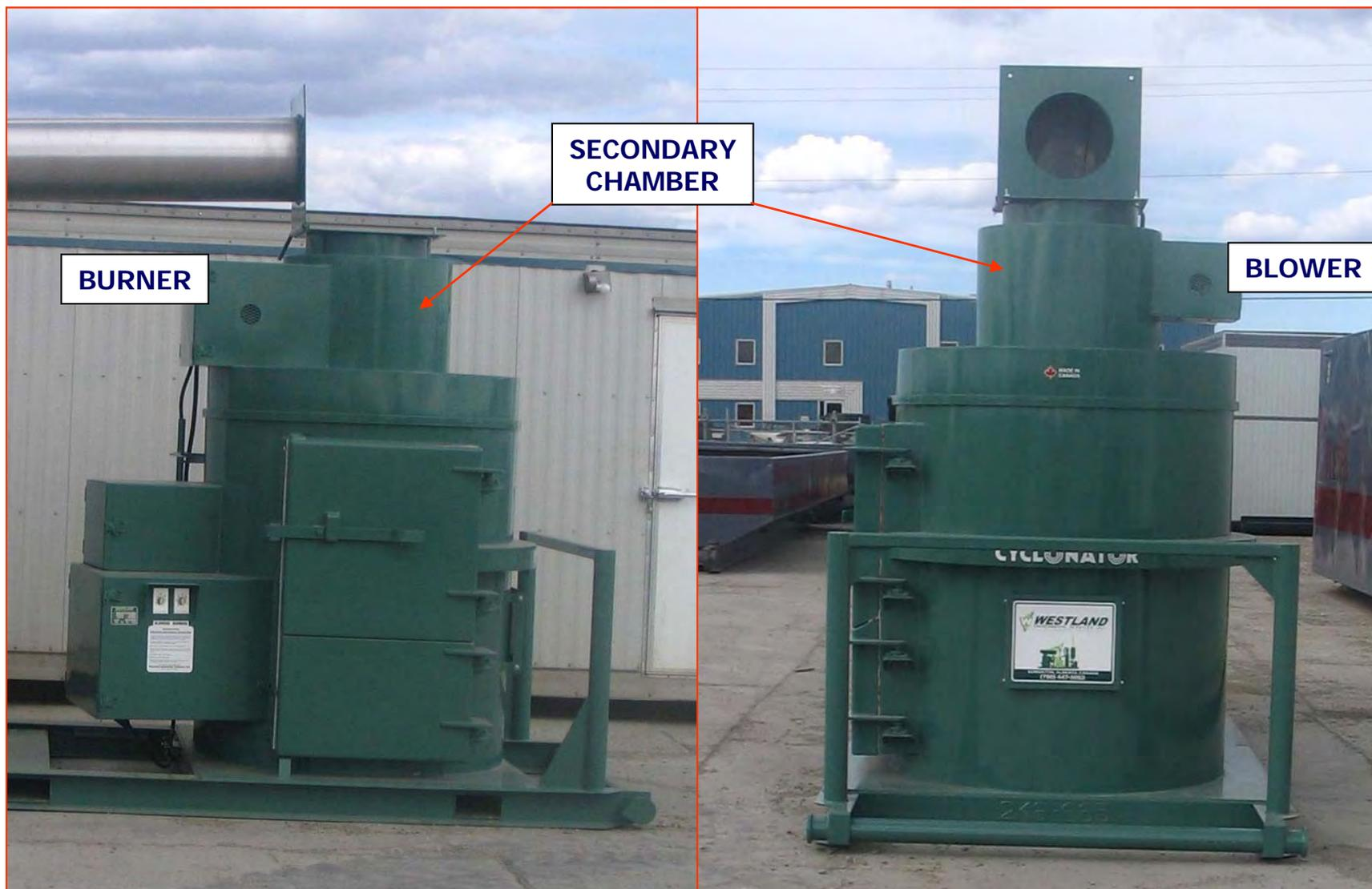
Figure 6 Photographs of the Dual-Chamber Design
