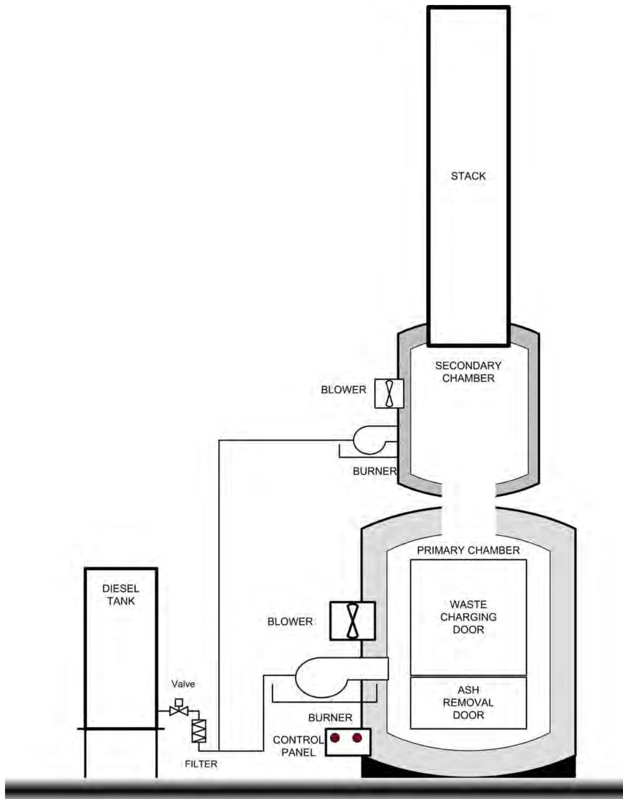
Figure 4 Schematic Diagram of Forced Air Dual-Chamber Design
