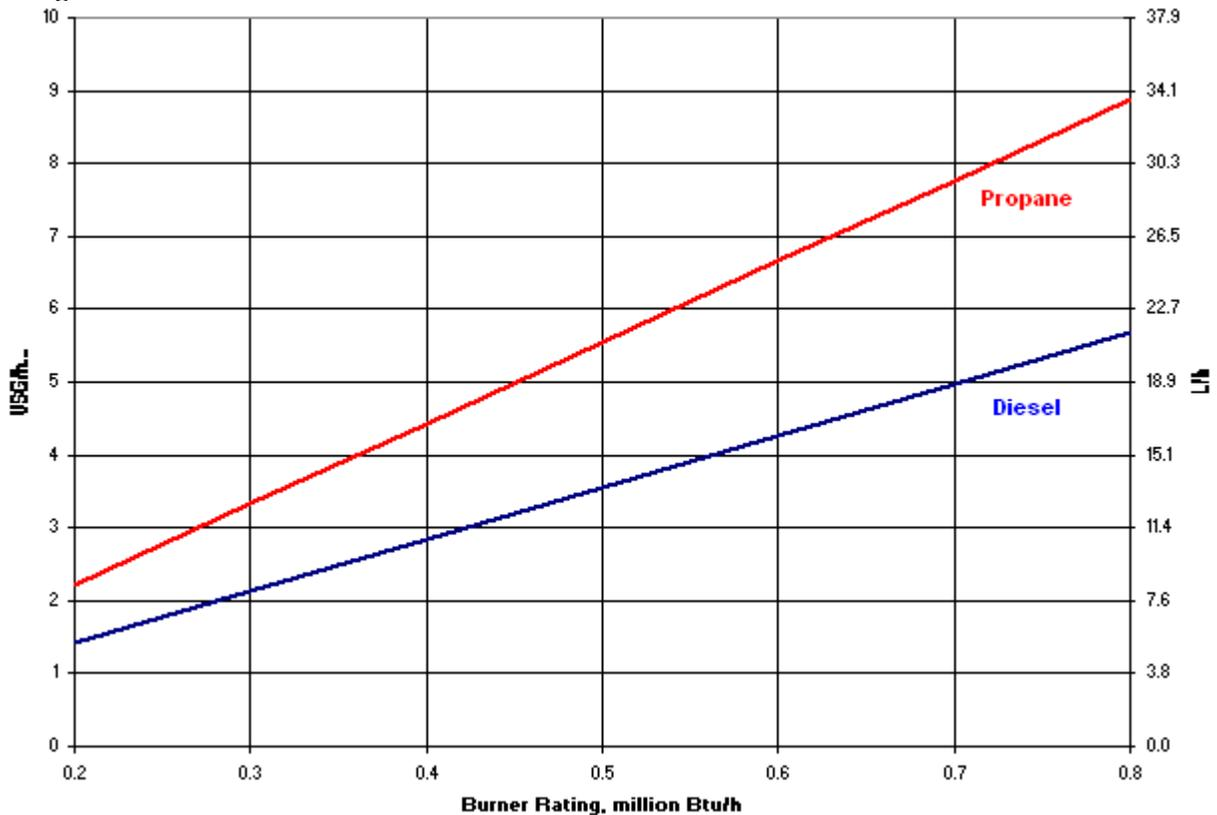
Figure 7 Consumption Rates of Propane and Diesel
