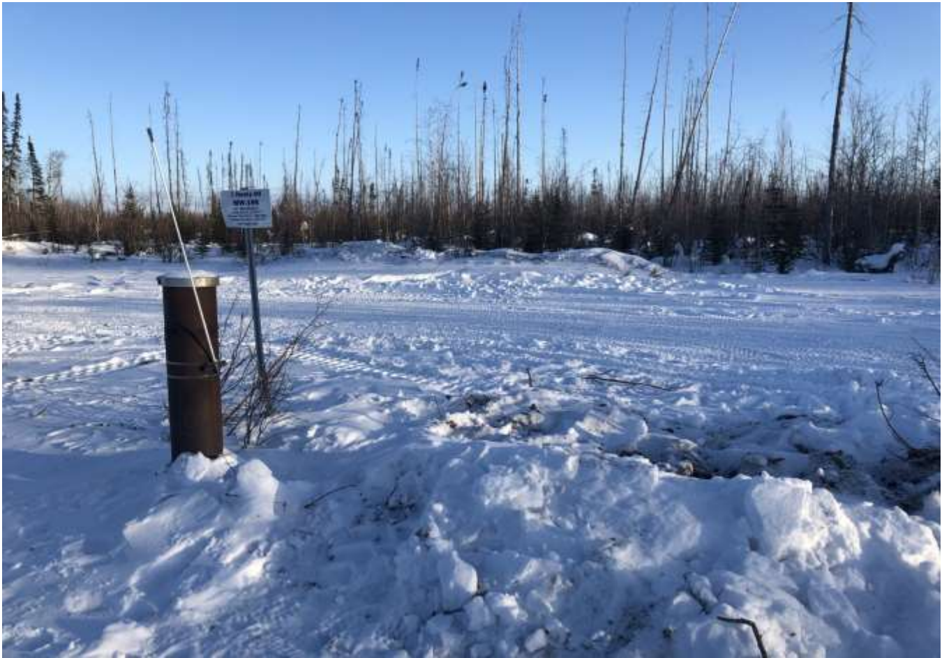
Figure 3 Groundwater monitoring well (MW-19B)
