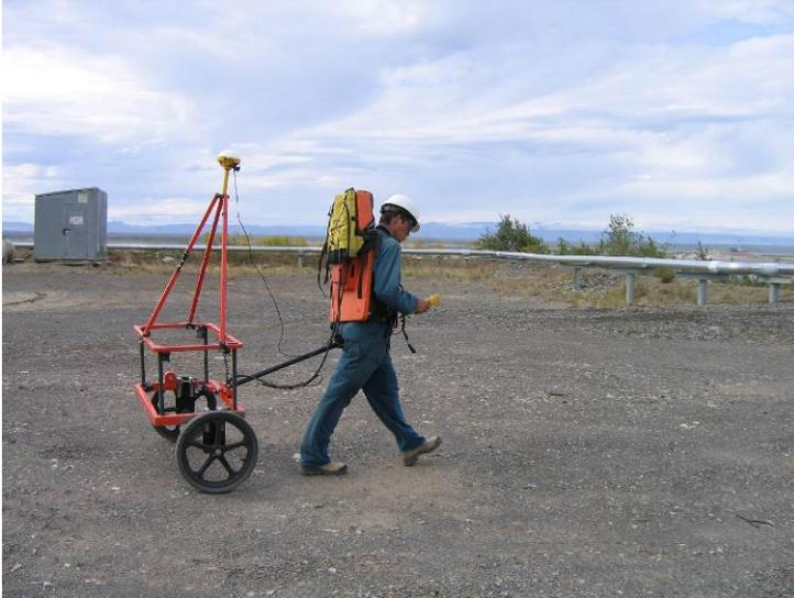
Overall, the research found that the geophysical surveys were successful in locating and/or confirming general locations of underground utilities (Imperial Oil 2008). This technology can be used to supplement traditional ground disturbance methods prior to initiating excavation work. Geophysical surveys are conducted regularly during abandonment and reclamation activities as part of site assessment activities at Norman Wells.
