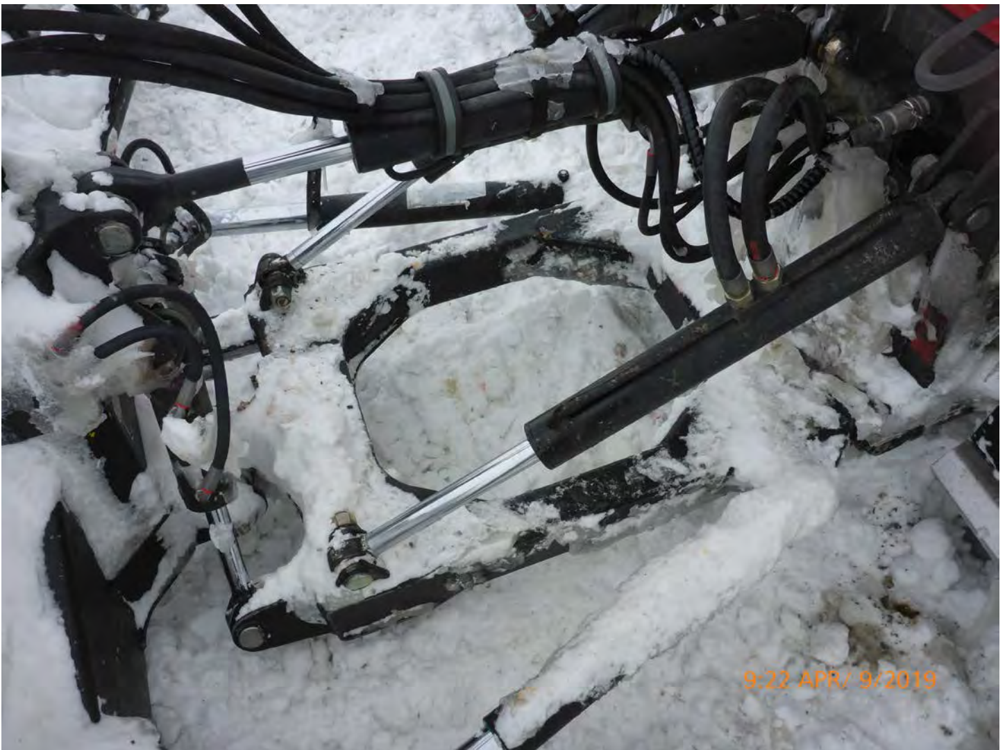
Photo 2 – Sable Haul Road – The Snow Cat had some small hydrocarbon drips and requires a drip tray as per Condition 37 of the Permit.
