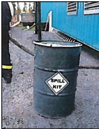
Figure 4 – Example of a spill kit kept nearby during fuel transfer operations
