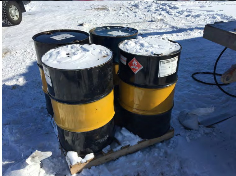
Photo #14: Fuel drums at the Bullmoose airstrip without adequate secondary containment.
