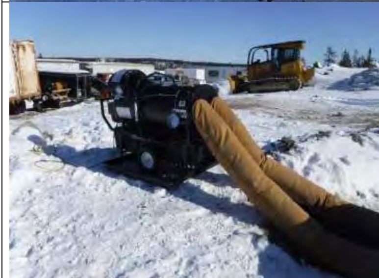
Photo #4: Frost Fighter at Alimak placed in secondary containment post inspection.
