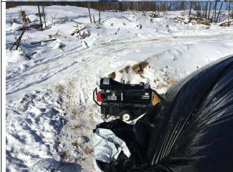
Photo #7: Frost Fighter at Mainway without secondary containment.
