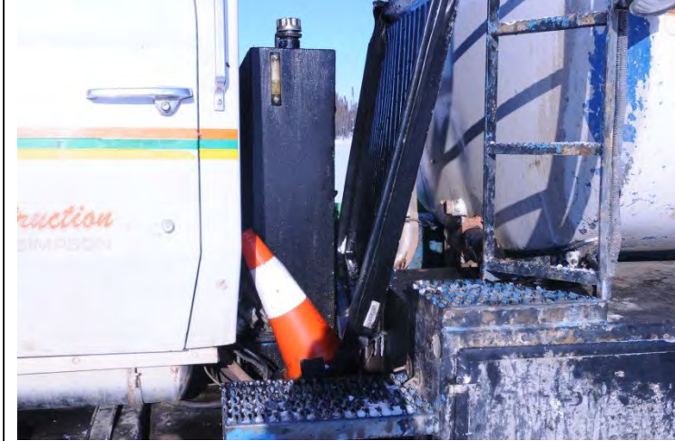
Photo #2. View of the back of the truck in Photo #1 showing hydrocarbon residue on the spill tray and spillage on the reservoir.
