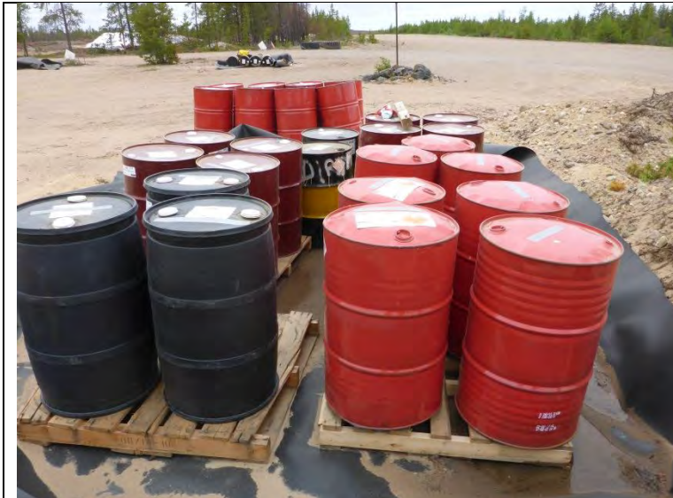
Photo #4: Barrels of fuel. Note the visible bulging of several drums.
