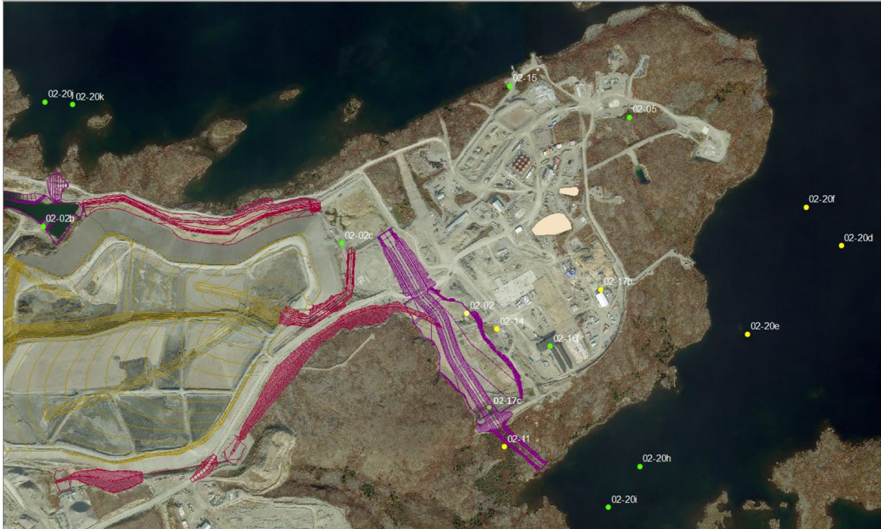
Figure 1: SNP Stations overlaid onto a 2023 satellite image of Snap Lake Mine with the design drawings for closure features. Yellow circles indicate stations to be discontinued. Green circles indicate stations to be retained .
