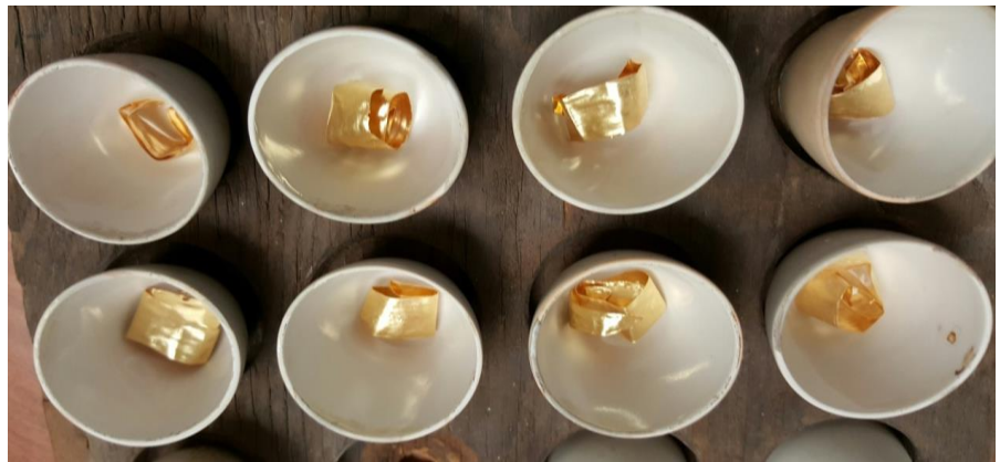
Picture 2. Au beads from fire-assaying of GF4-GF7 pan conc.
