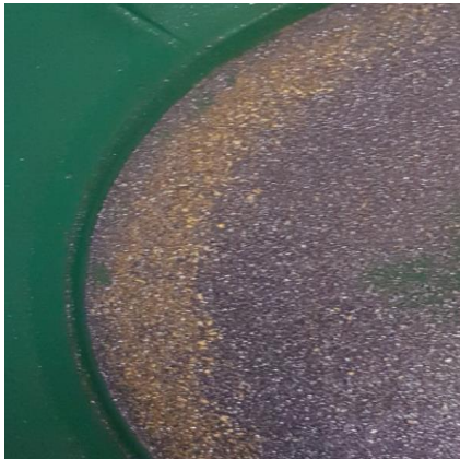
Picture 1. Panning of GF4 gravity concentrate
