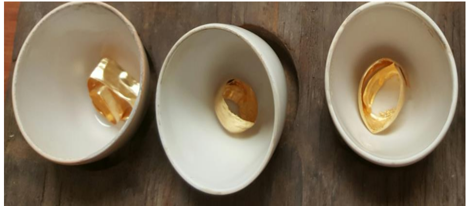
Picture 2. Au beads from fire-assaying of GF1-GF3 pan conc.
