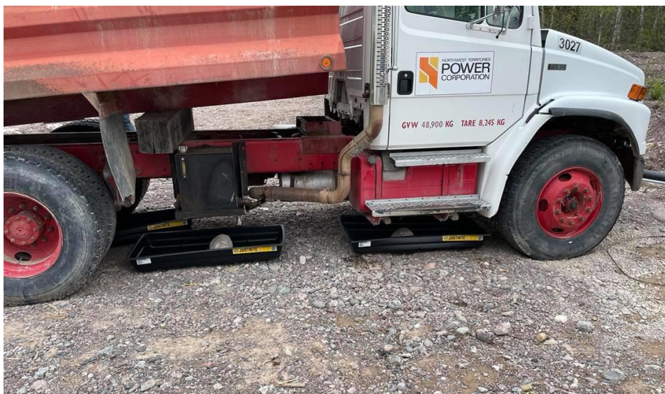
Figure 1 – Drip tray deployed under parked equipment
