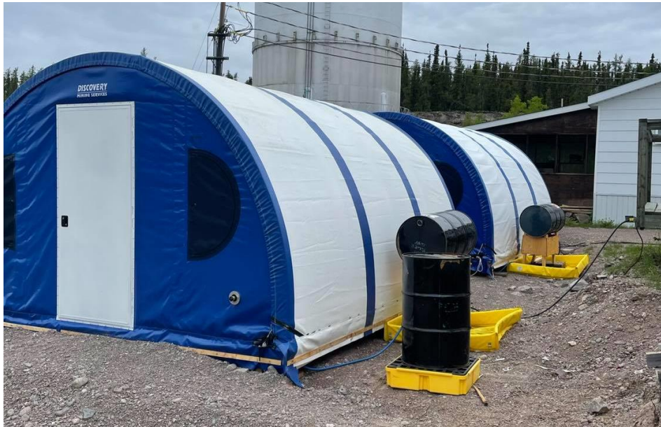
Figure 3 - portable secondary containment under individual drums
