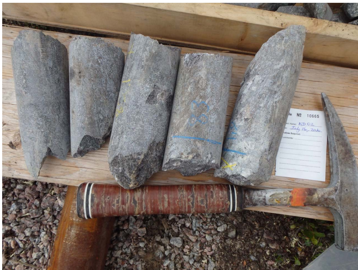
Figure 3. A typical sample collected for geochemical testing from drill core representing the proposed decline.
