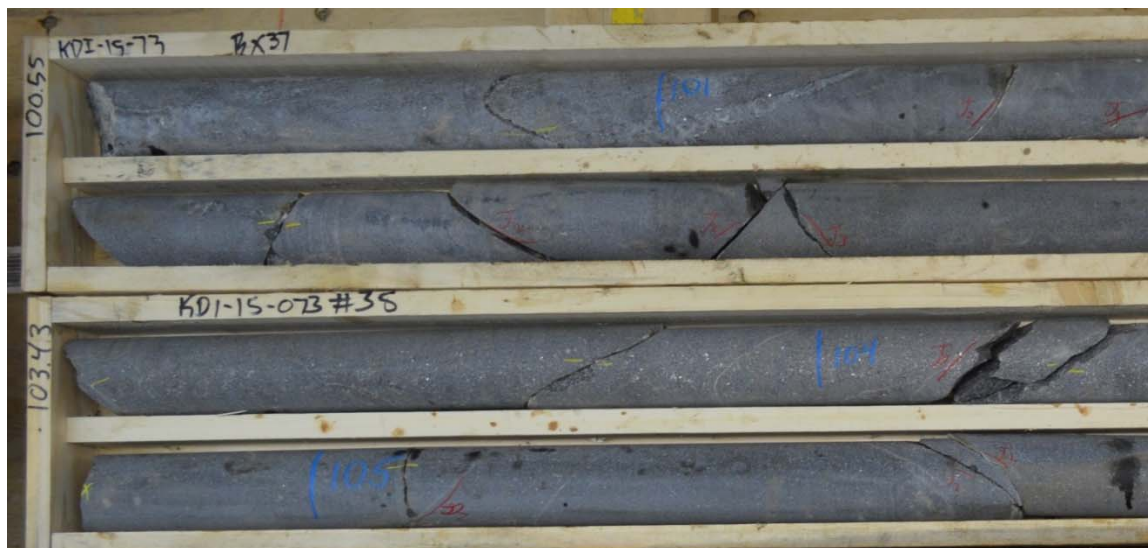
Figure 5. Drill core from hole KDI15-073 showing relatively homogenous metagreywacke.
