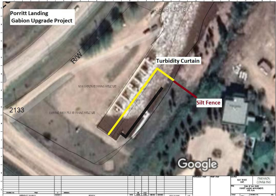
Figure 2- Turbidity curtain and silt fence for gabion upgrades
