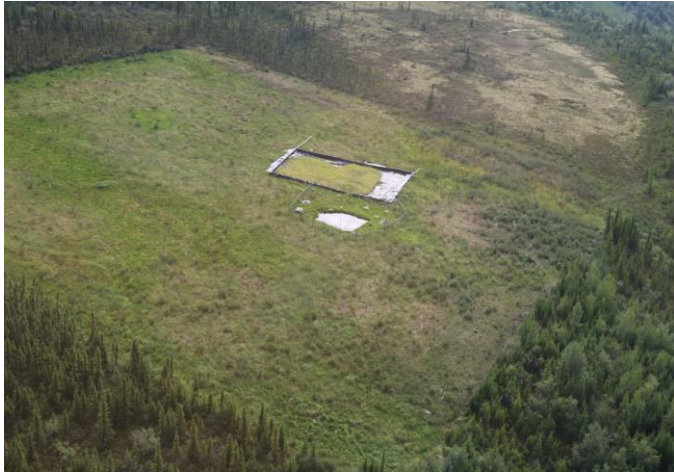
Figure 3 Photo showing water pooling at well center due to contaminated material being removed and placed in berm.
