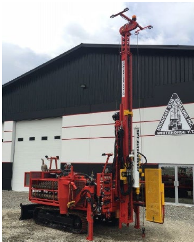
Photo 1. Proposed Multi-Power Locust Auger/Air Rotary/RC Drill Rig
