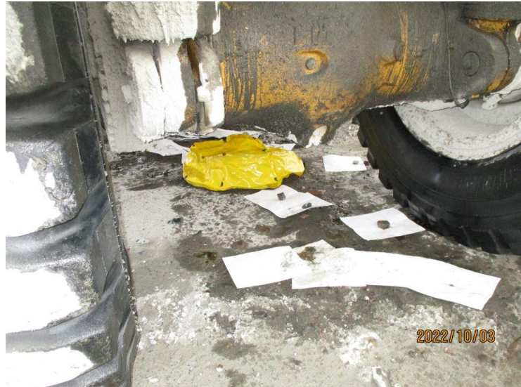
Photo 1: South Sable Waste Rock Storage Area – view of flexible spill tray and pads deployed under 7490 haul truck.
