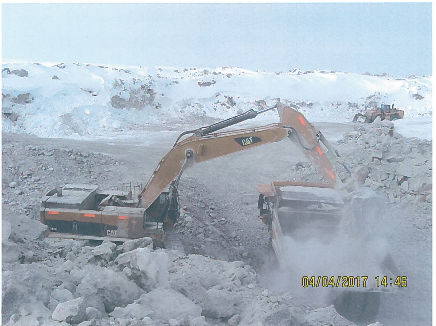
Photo 2: Sable Quarry Pit - Clean granite is being excavated from the Sable Quarry Pit and being stock piled near the crusher pad for future construction projects
