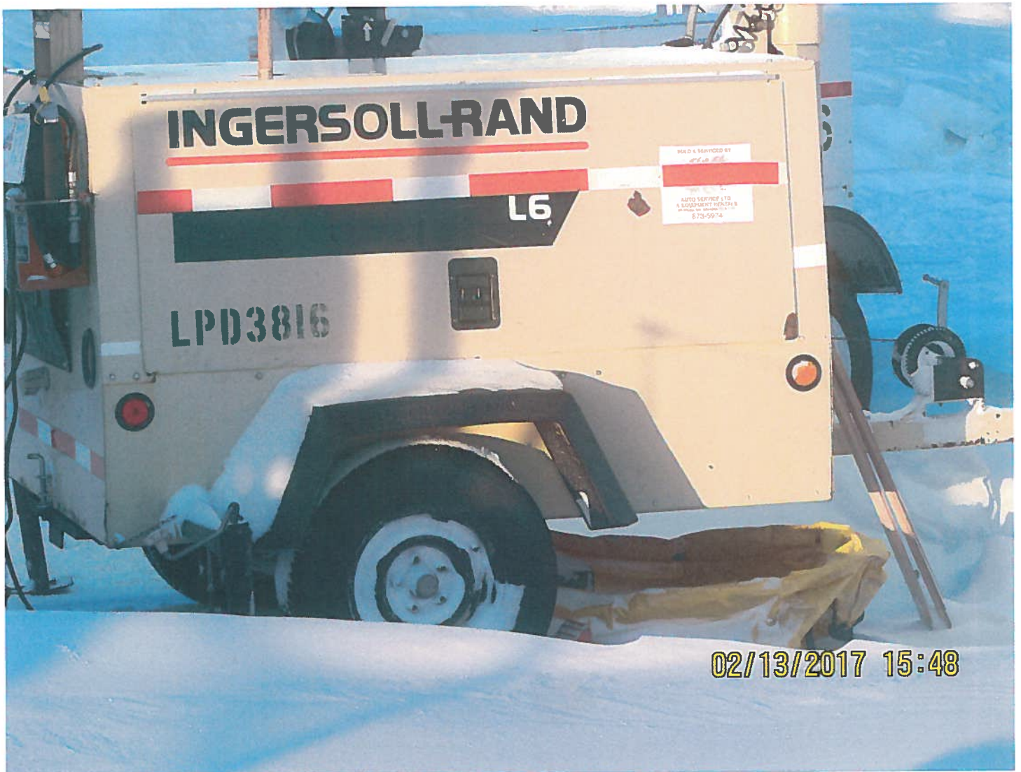
Photo 7: Sable Development/Sable Lake- All stationary equipment had drip trays placed under the engines
