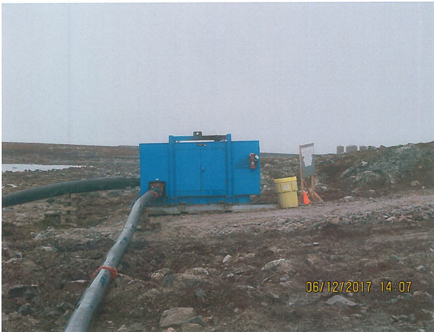
Photo 3: Sable Lake - A dewatering Pump was set up at Sable Lake to remove water from Sable to Ulu Lake. The pump is in secondary containment and a Spill kit was in close proximity.
