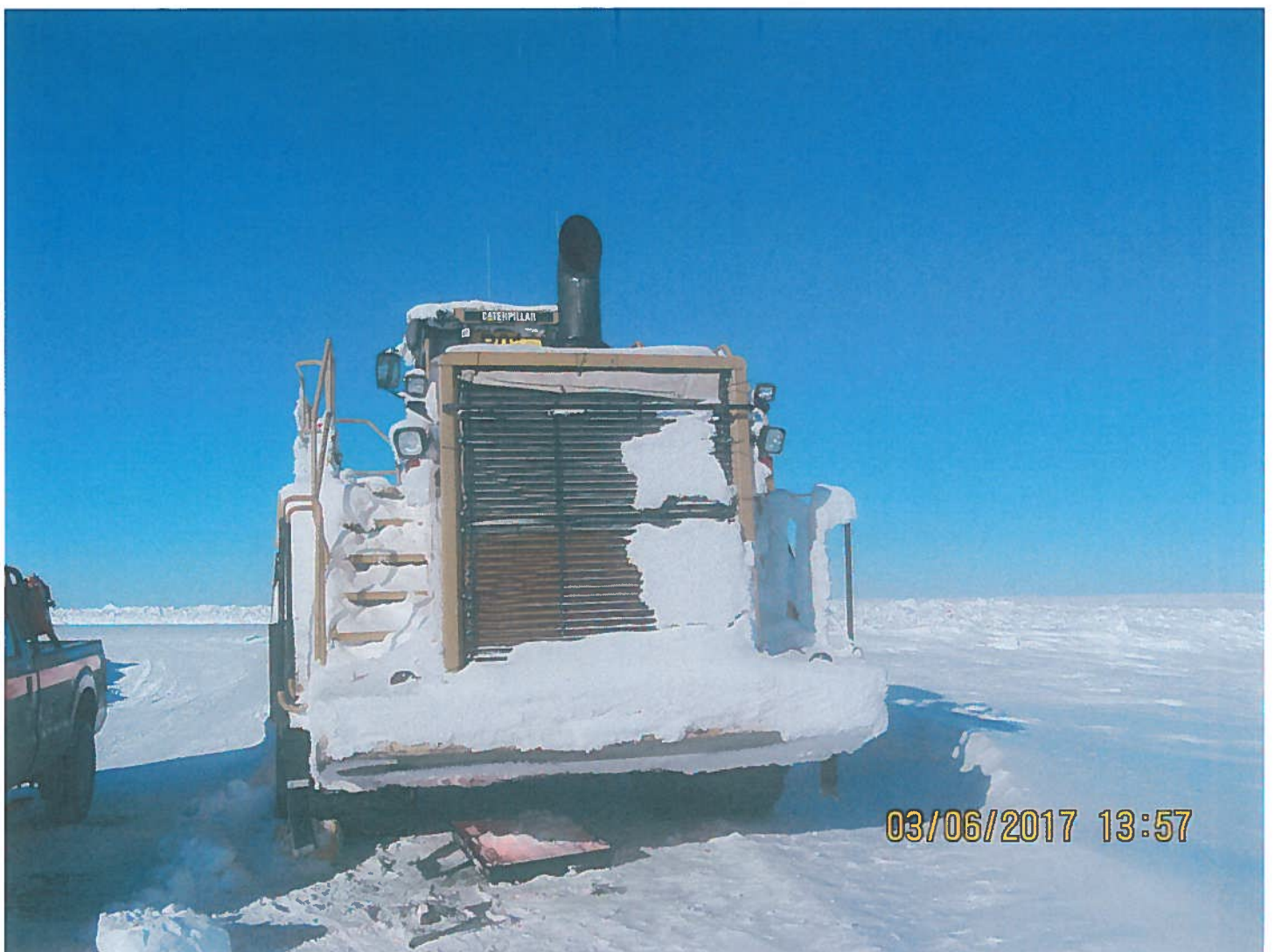
Photo 2: Falcon Lake Road - A loader ( R015 988 ) was located on the Falcon Lake access road. Repair work will be conducted shortly. Glycol spill will need to be disposed of to an approved facility.
