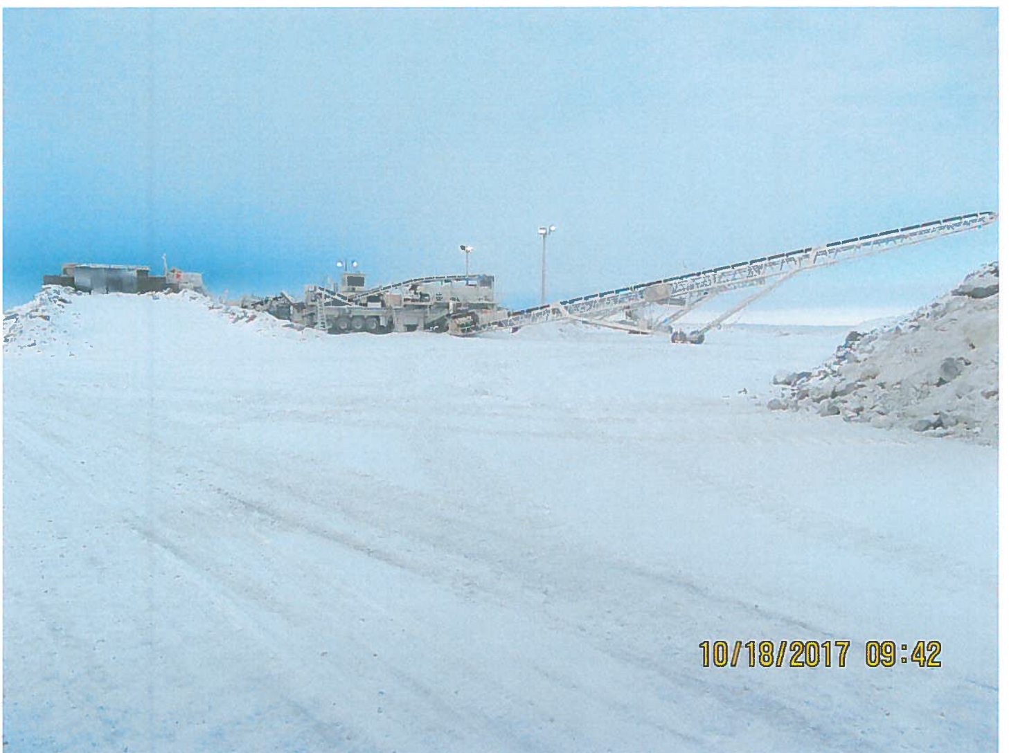
Photo 4: Sable Crusher Laydown Area - A crusher from the Misery facilities was relocated to the Sable Crusher pad. The crusher will be producing clean granite material required for stemming.
