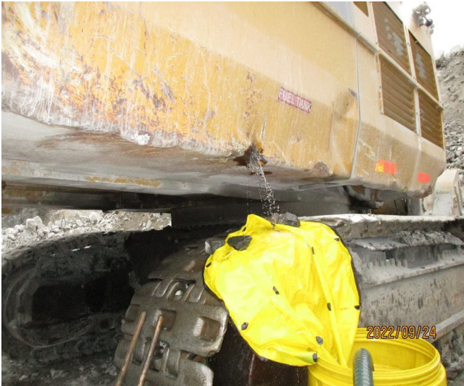
Photo 1: Sable Pit – Containment barrel with vacuum pump to catch leaking diesel from impact site on shovel.
