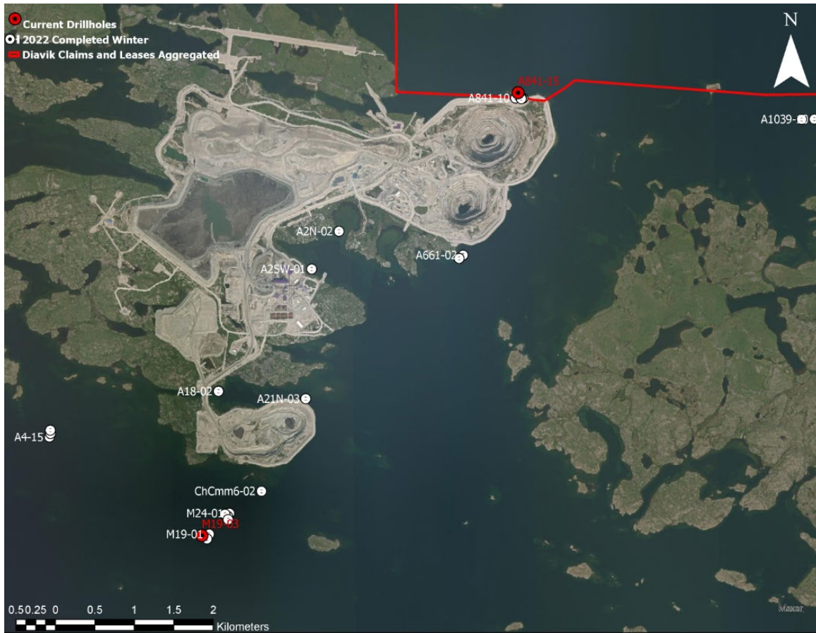
Figure 1: Plan map showing the completed holes for the month of April – white circles for completed holes, and red circles for in progress holes.
