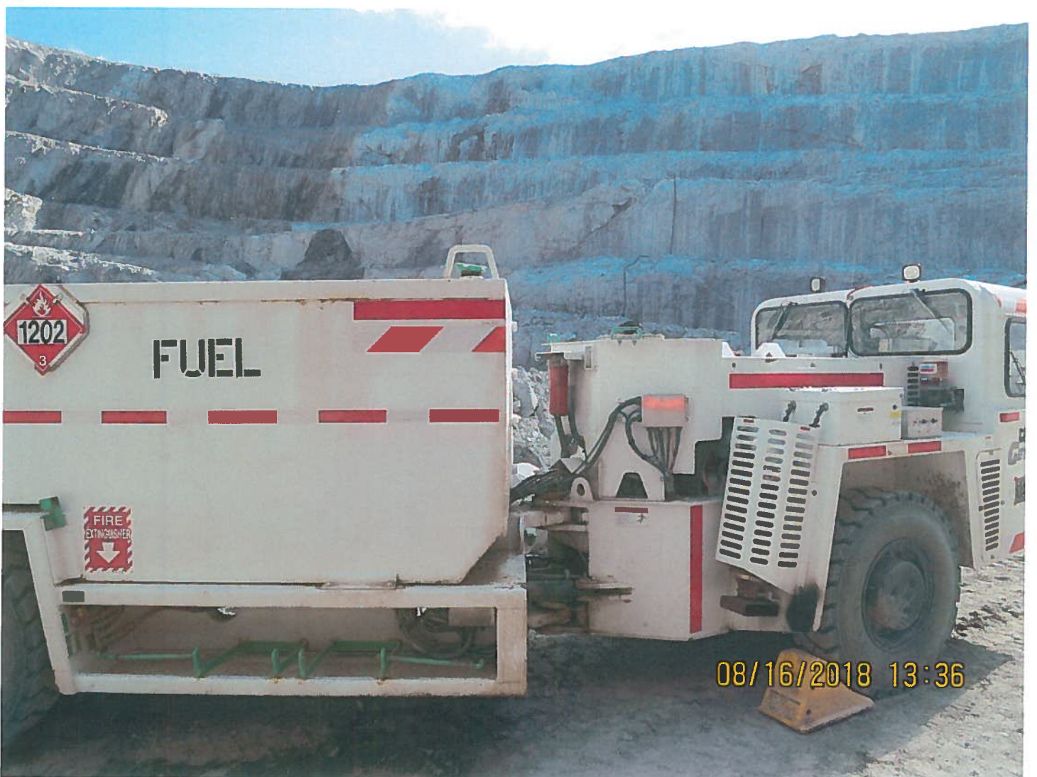
Photo 16: 2235 portal - All vehicles that will be used in the underground project will be fuelled by a mobile fuel truck.
