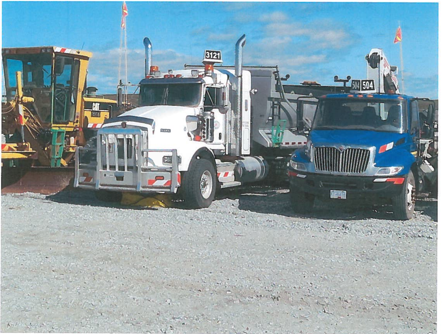
Photo 21: Misery Pit Laydown Area - several pieces of Equipment were placed in the Misery Pit Laydown. All stationary equipment had drip trays installed under them to catch drips.
