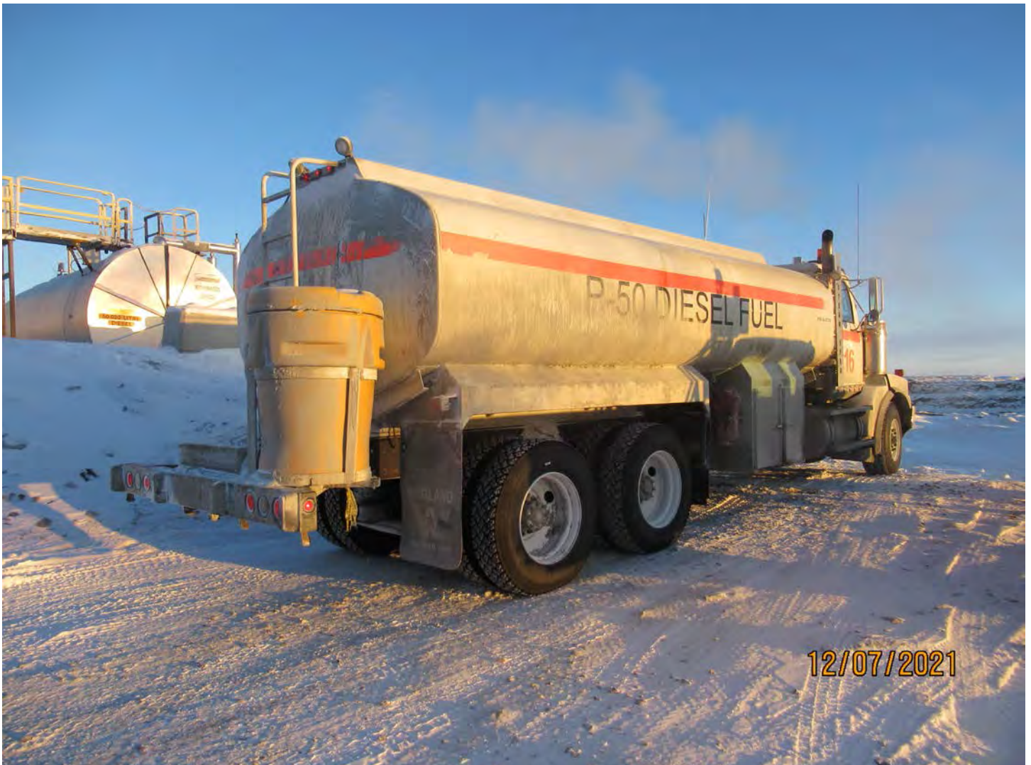
Photo 6: This fuel truck was transferring fuel to the fuel tank in Photo #5. Note the onboard spill kit.
