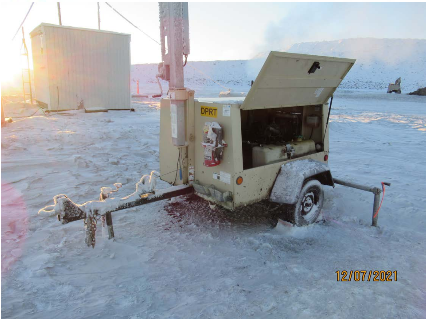
Photo 11: A second operational light plant at the ore laydown that requires secondary containment.
