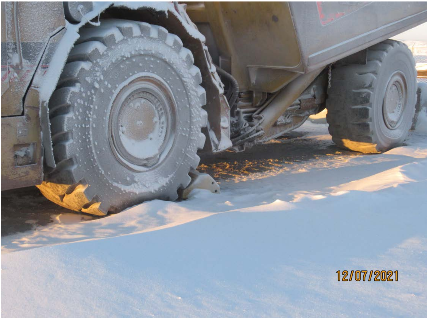
Photo 30: The Permittee must ensure secondary containment is used under parked equipment and is properly maintained.
