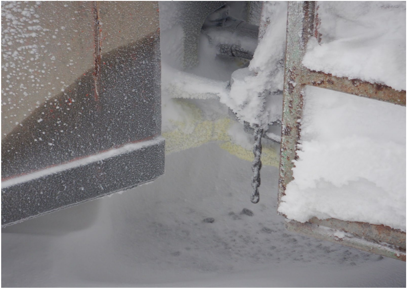
Photo 9 – Misery surface – Laydown – Fluid leakage from vehicle #03498
