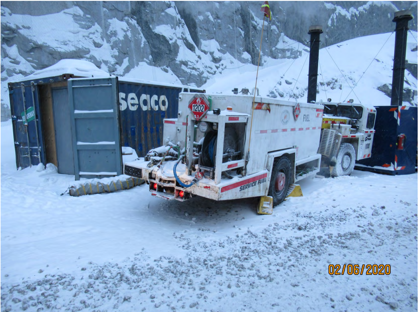
Photo 15: There was no secondary containment in place under this Getman on the 2235 Lower Portal ramp.
