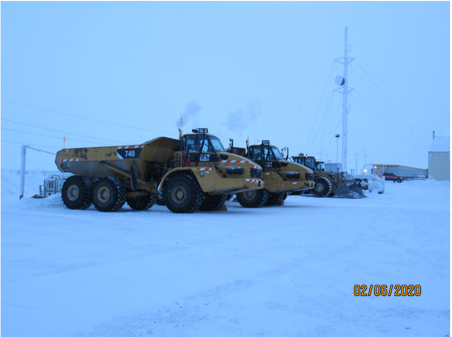
Photo 19: There was no secondary containment in place under this parked equipment on the east of Misery Camp.
