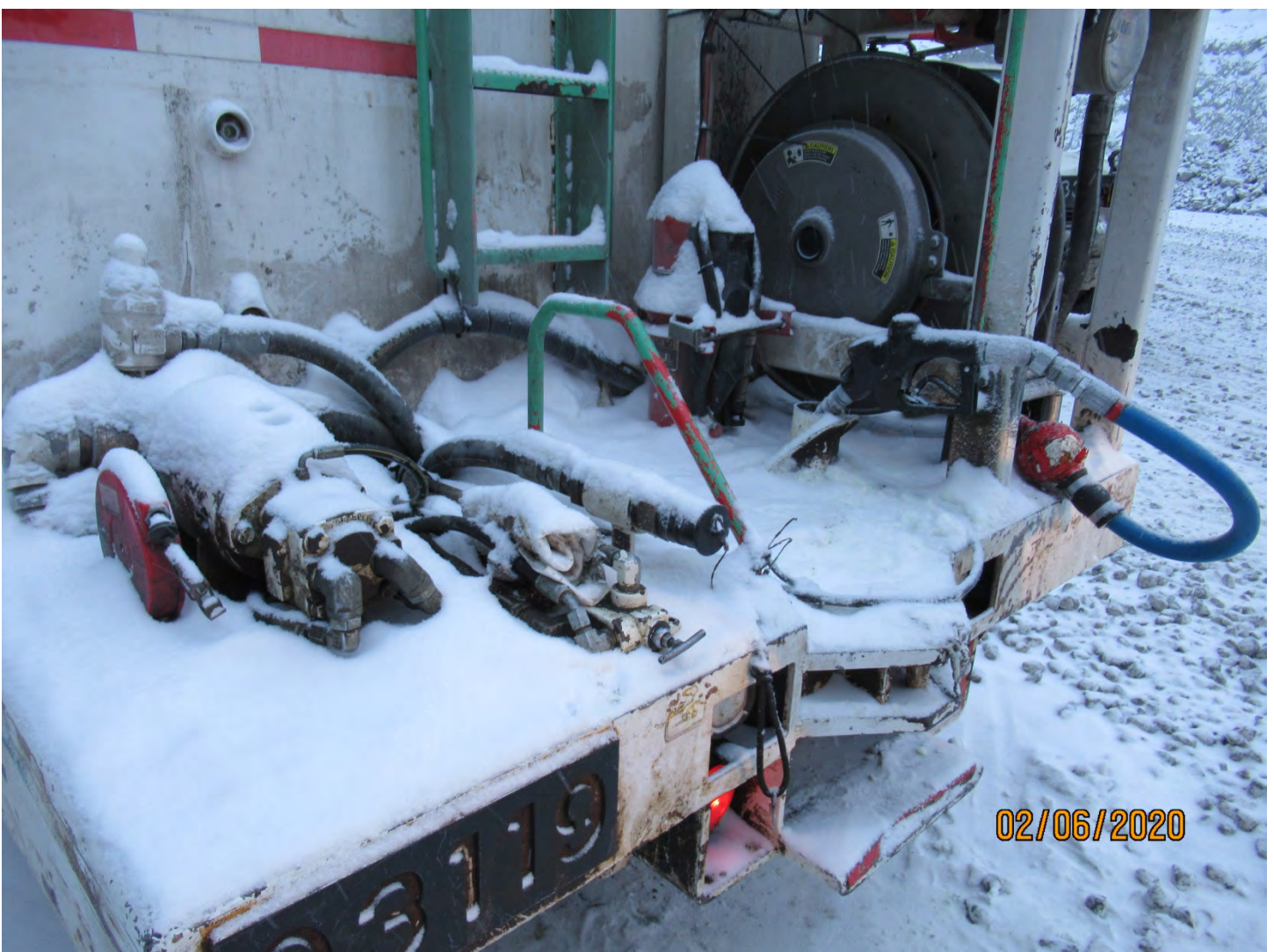
Photo 16: Though the fuel nozzle was stored in containment when not in use, it appeared secondary containment was not being used during fuel transfers at the Getman.
