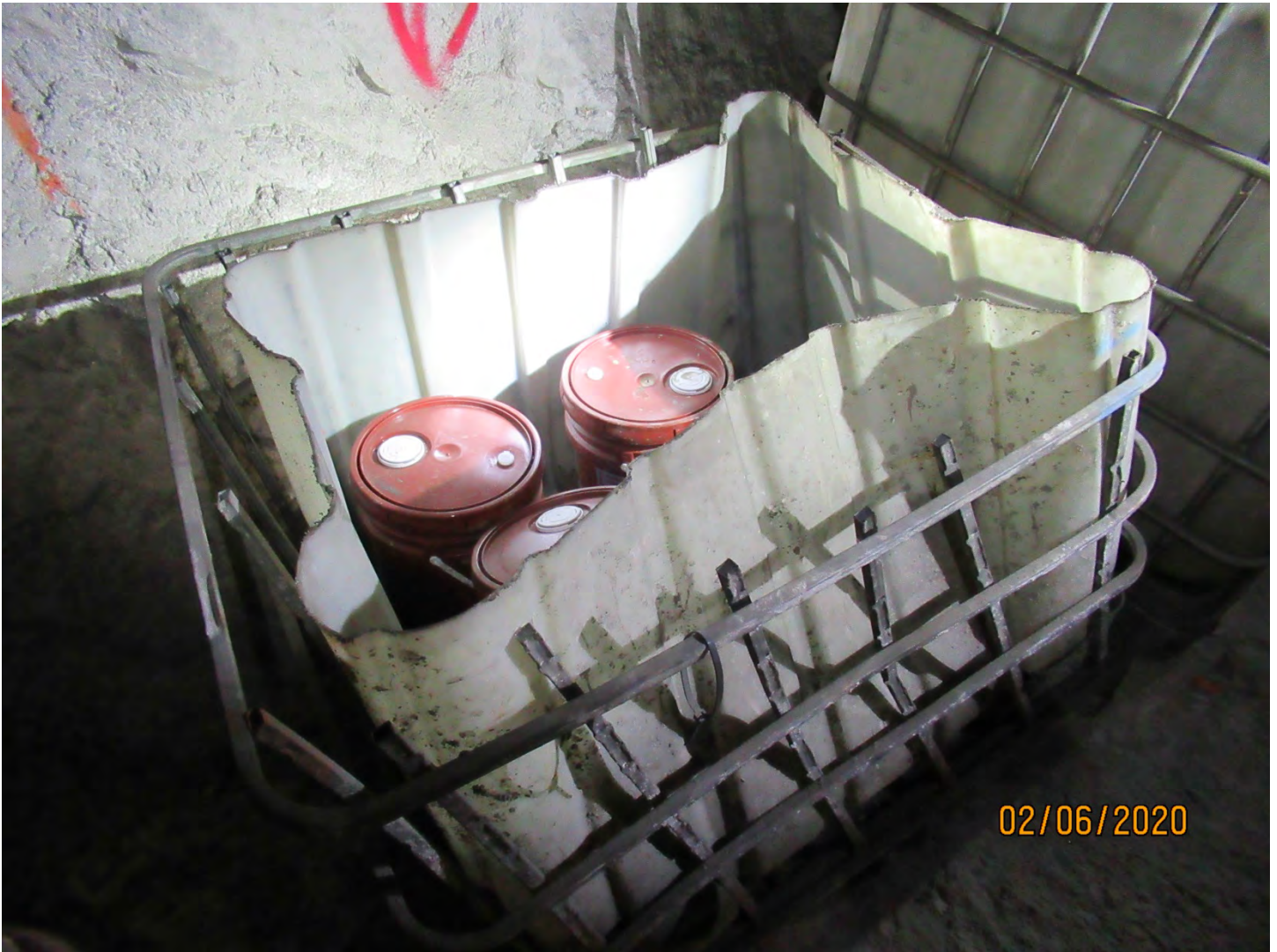
Photo 13: Hydrocarbons at the UG were properly staged and within secondary containment.
