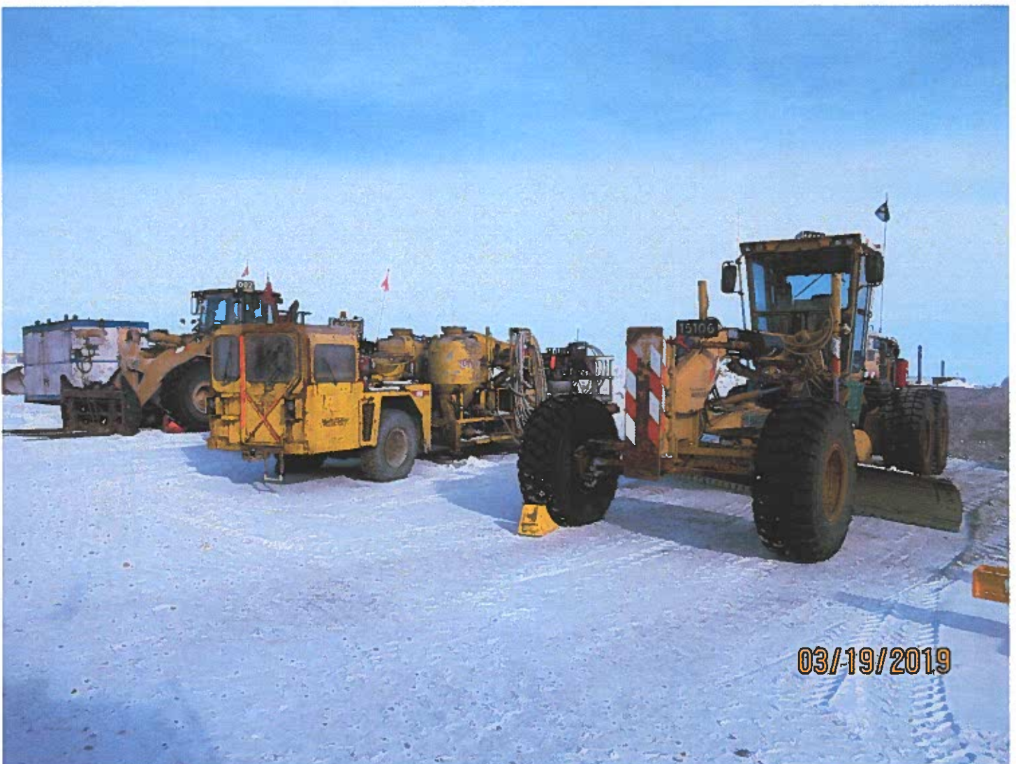
Photo #22 - W2017D0004 MUG Project Equipment parked for two hours or more requires secondary containment.
