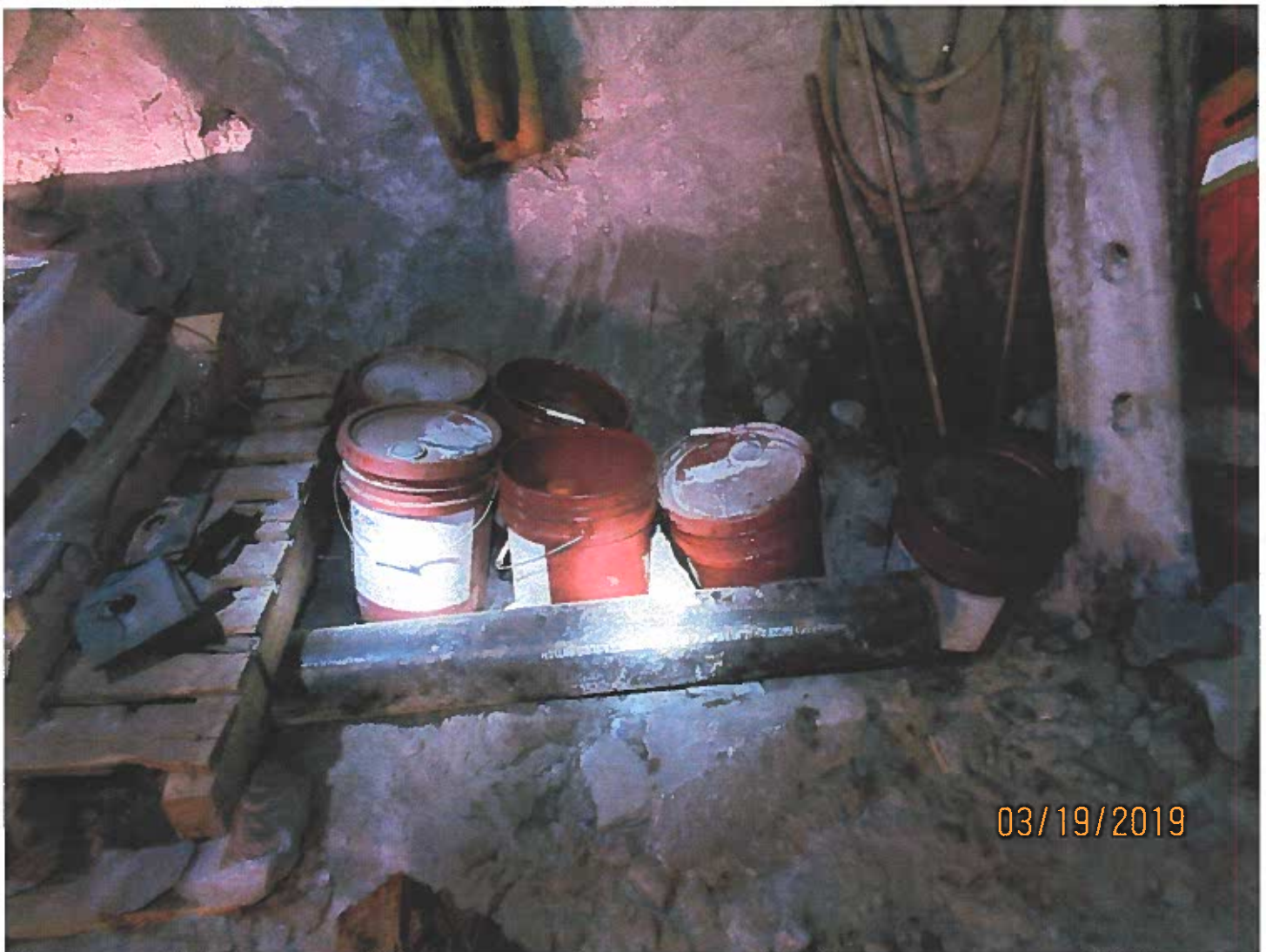
Photo #6 - W2017D0004 MUG Project Hydrocarbons were being staged out of containment on the 2175 Level.
