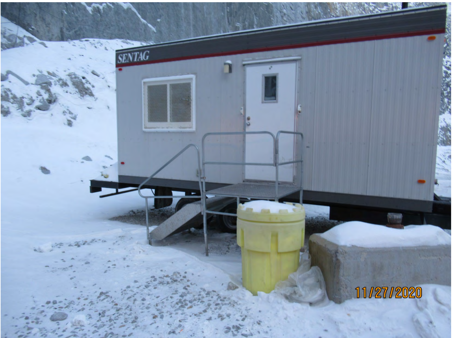
Photo 10: Spill response materials were readily available at the washroom building on the 2235 Lower Portal ramp.
