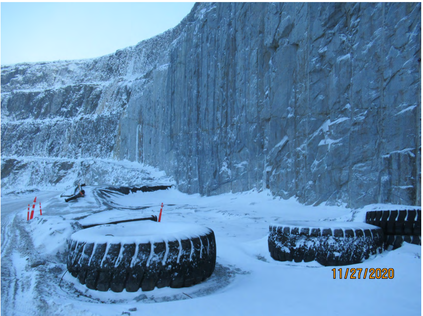
Photo 2: A water sump has been established downgrade and adjacent to the 2340 Upper Portal.
