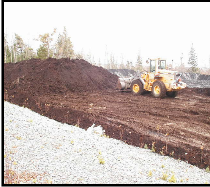
Figure 7. Solid waste residual drying beds (Lake Major WTP, Dartmouth, NS) (M. Walsh, 2014)
