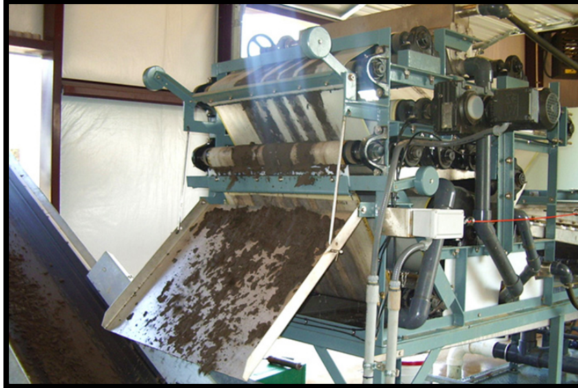
Figure 10. Solid waste dewatering by a belt filter press (Phoenix Process Equipment, 2018)
