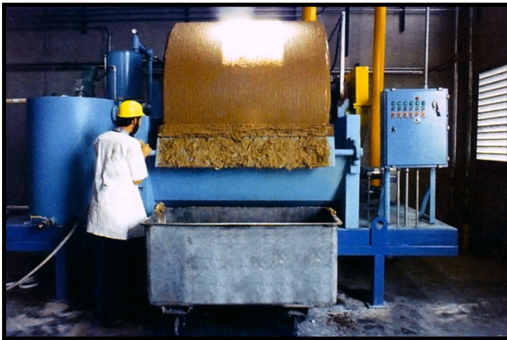
Figure 8. Solid wastes dewatering by a vacuum drum filter (WesTech Engineering Inc., 2020)
