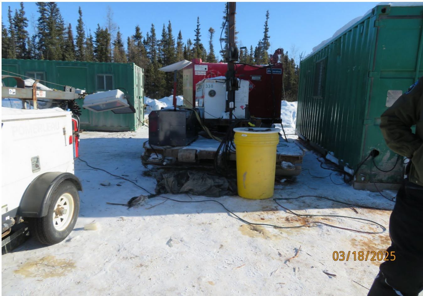
Figure 6 Spill response material is readily available and visible in areas of fuel handling.
