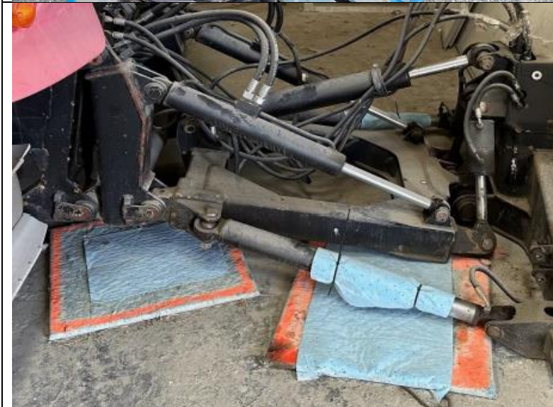
Photo #10: Photo submitted by on-site staff to demonstrate compliance of updated secondary containment measures applied to machinery.
