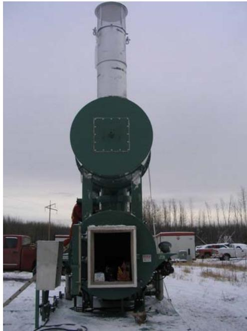
Figure 2.2 Typical Controlled Air Dual Chamber Incinerator
