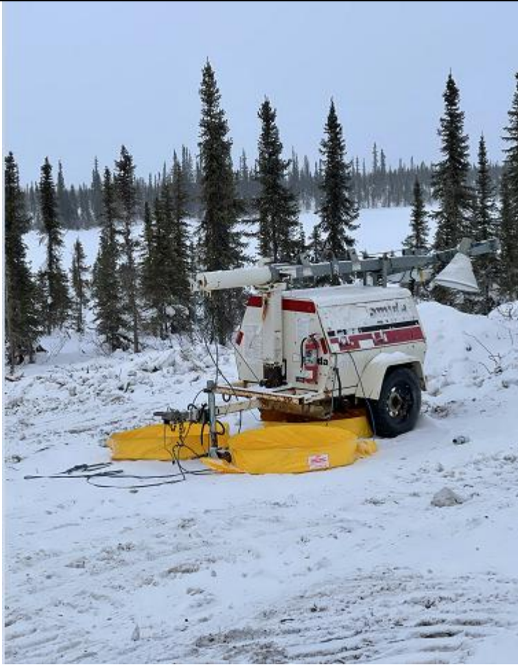
Drip Trays on Site
