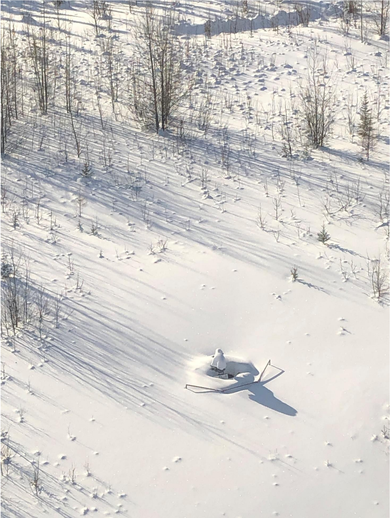
Photo #2: Aerial view of Arrowhead River O-38 Well Head – No wind indicator
