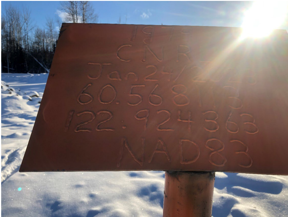
PHOTO #1: Well abandonment sign
