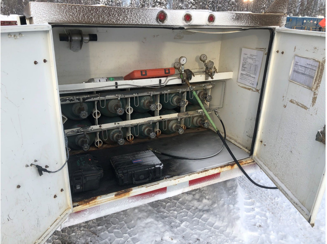
Photo #11: Supplied Air trailer on site during well abandonment operations.
