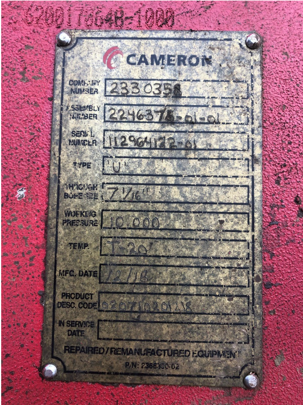
Photo# 13: Double gate placard confirmed to match BOP certification previously provided to OROGO.
